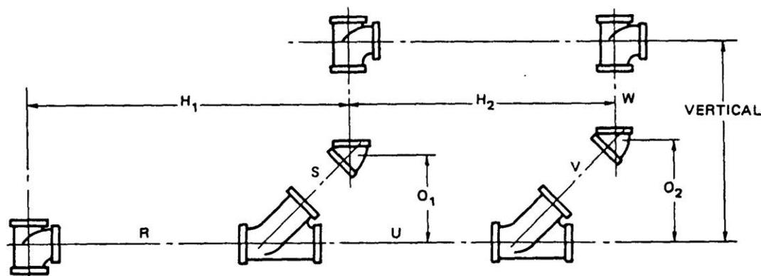
18. What is the end to end length of pipe W if  $H_1$  measures  $4'-7\frac{1}{2}"$ ,  $H_2$  is  $3'-4"$ , the vertical measure is  $5'-11\frac{1}{2}"$ , and each offset is  $10"$  for an assembly using  $2"$  threaded pipe?
